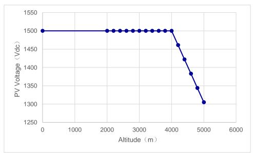
DC Voltage Curve VS. Altitude of SUN2000-300KTL-H1
