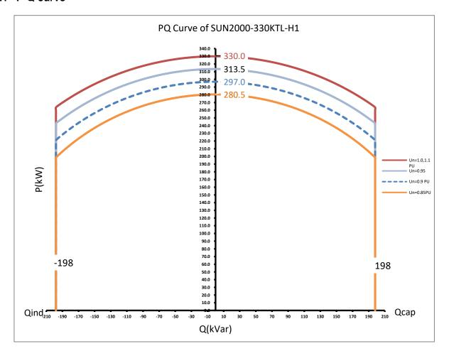
For SUN2000-330KTL-H1 inverter, its rated AC active power is 300kW and maximum AC active power is 330kW, maximum apparent active power is 330kVA,maximum reactive power range is - 198kVar~+198kVar.
