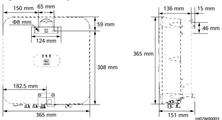
Figure 4-7 Mounting bracket dimensions
