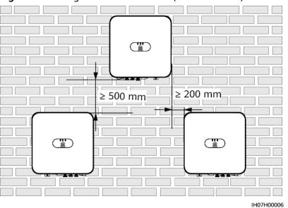
Figure 4-4 Triangle installation mode (recommended)
