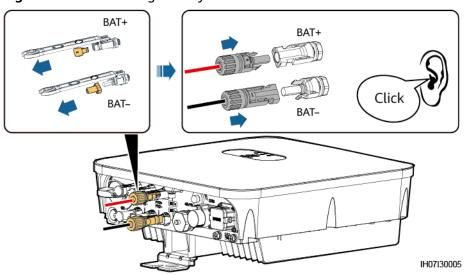
Figure 5-17 Connecting battery cables
