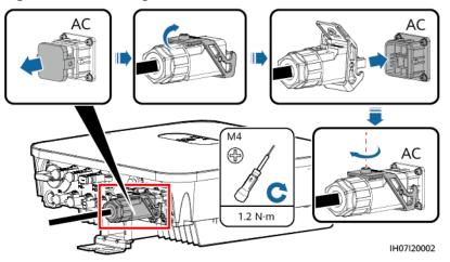
Figure 5-10 Securing an AC connector
