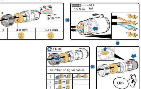
Figure 5-25 Assembling a signal connector (single SUN2000)
