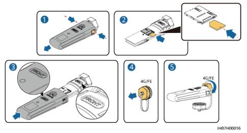
• WLAN-FE Smart Dongle (FE Communication)
