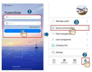
**Step 2** Connect to the solar inverter WLAN and log in to the device commissioning screen as the **installer** user.
