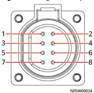
Figure 5-18 Signal cable ports
