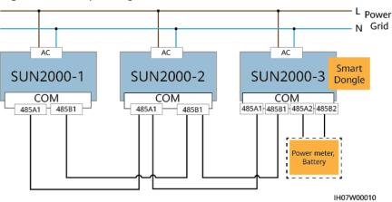
Figure 5-21 In-phase grid connection
