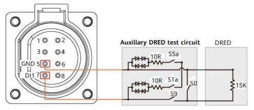
Figure 7-17 Wiring diagram for the DRM function
