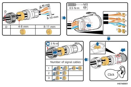
**Step 2** Connect the signal connector to the corresponding port.
