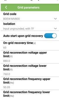
Figure 7-4 Power grid parameters (special user)
