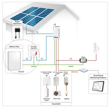
Figure 1: SolarEdge System with Device Control
