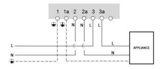
Figure 5: Connecting to appliance
