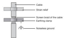
Fig. Shielding procedure at cabinet entry.
