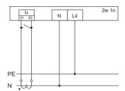
Fig. Measurement of the voltage between N and PE. Measurement of the current in the neutral conductor.
