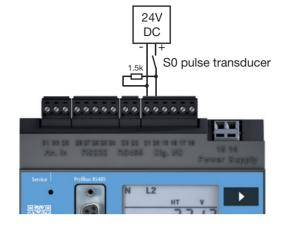
Fig. UMG 604-PRO with inputs for 24V. Example with S0 pulse transducer.
