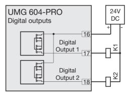
Fig. Connection of a DC voltage relay to the digital outputs.
