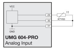
Fig.42.1 Example, temperature measurement with a KTY83.
