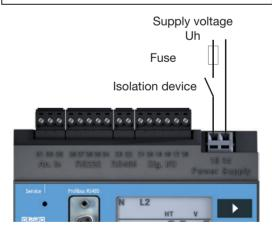
Fig.23.1 Example connection for the supply voltage Uh.
