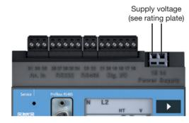
Fig.23.1 Example connection for the supply voltage Uh.
