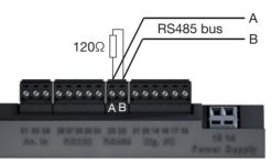
Fig. RS485 interface, 2-pin plug contact with termination resistor (item no. 52.00.008).
