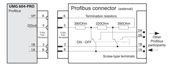
Fig. 36.1 Profibus connector with termination resistors.
