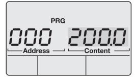
Fig. UMG 604-PRO display in programming mode
