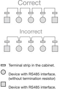
(with termination resistor on the device)
