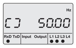
Fig. Display example for rotation field and frequency.
