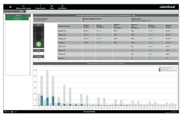
Fig. IEC 61000-2-4 parameters with traffic-light principle
