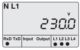
Fig. Display example for "Display mode". Measured value indication  $U_{11N} = 230.0 V$ .
