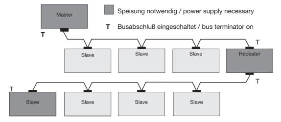
Fig. Bus structure illustration
