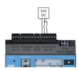
Fig. Connection example of digital inputs.
