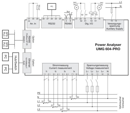
Fig. Connection example for UMG 604-PRO
