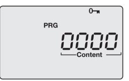
Fig. Request window for the display password
