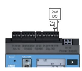
Fig. Connection example of digital outputs.
