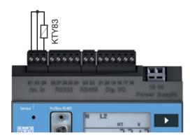
Fig. Connecting temperature sensor to the measurement input
