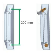
Drill wall holes with a suitable drill in accordance with the building inspectorate approval for the frame anchor. For each socket 2 holes, 80 mm deep 10 mm, must be drilled. Then anchor the dowels through the socket up to the collar in the holes and screw in the screws.
