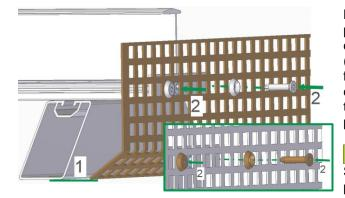
Mount the perforated plate with the angled leg pointing under the module field, flush with the lower or upper perforated plate and resting on the wall (1). Place the long leg on the adapter plate and fasten it with the two self-drilling screws with countersunk washer to the left and right edge of the adapter plate through the openings of the perforated plate (2).
