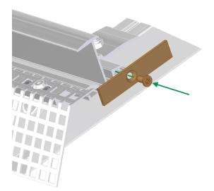
Place the adapter plate with the longer side of the leg pointing upwards on the end of the insertion rail and screw it into the screw channel of the insertion rail with the countersunk screw included in the set. Align the adapter plate parallel to the bottom of the rail and fix it flush with the upper and lower perforated plate.
