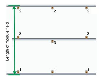
For the top and bottom insertion rail of the module array, the cross rail connector set N IR is mounted on the inside of each (1, 2).
