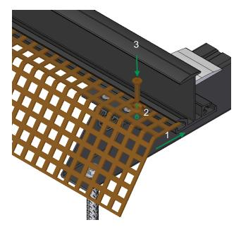
For the attachment of the upper perforated plates, slip guards must also be mounted on the uppermost base as described above.
