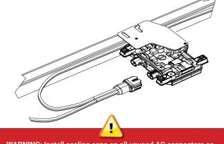
WARNING: Install sealing caps on all unused AC connectors as these connectors become live when the system is energised Sealing caps are required for protection against moisture ingress.
