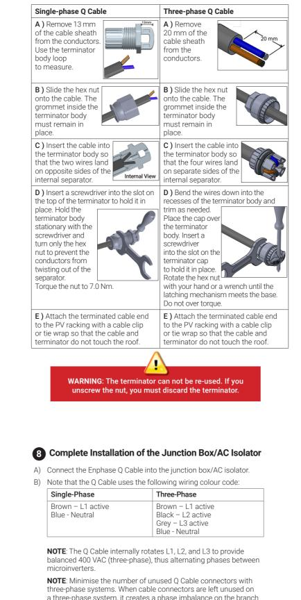
a three-phase system, it creates a phase imbalance on the branch circuit. If multiple cable connectors are skipped over multiple branch circuits, the imbalance can multiply.
