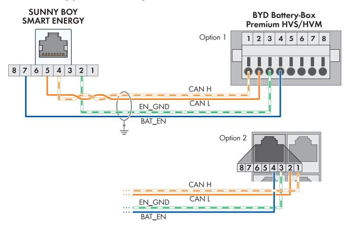
Figure 1: Cabling plan Sunny Boy Smart Energy with Battery-Box Premium HVS/HVM
