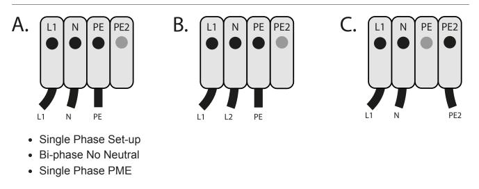
(UK only) can be connected to the PME supply according to BS7671:2018amd1:2020 722.411.4.1
