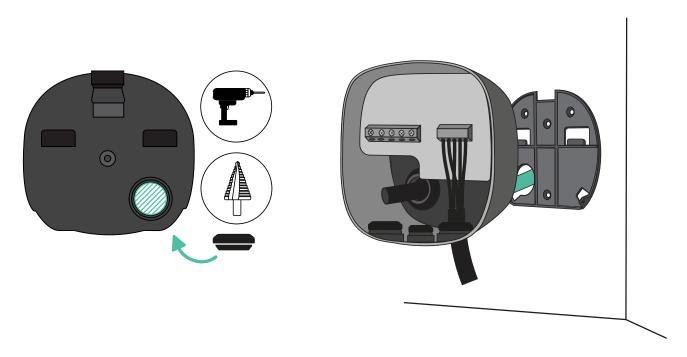
Fix your charger to the wall plate and then fix it using the appropriate screws.
