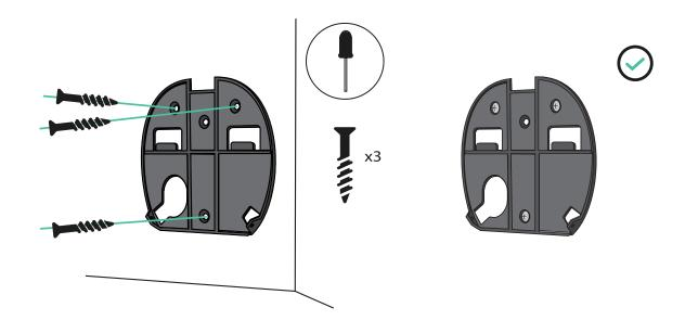
If case power supply wiring comes from the wall, ensure to place the wires through the wall plate hole before fixing the wall plate.
