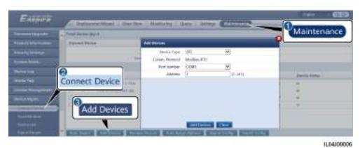
ParameterDescriptionDevice TypeSet this parameter to STS.Port numberSet this parameter to the number of the COM port connected to the STS.AddressSet this parameter to the communications address of the STS.
