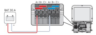
Figure 24: Overview for connection of one battery with a charging/discharging current limit of 30 A
