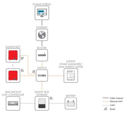
Figure 7: Design of system communication
