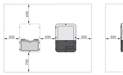
Figure 13: Recommended clearances(Dimensions in mm)
