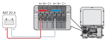
Figure 23: Overview for connection of one battery with a charging/discharging current limit of 20 A
