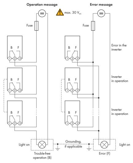
Figure 16: Circuit diagram with multiple inverters for connection to an operation indicator and circuit diagram for connection to a fault indicator (example)
