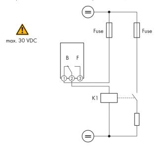
Figure 17: Wiring diagram for connection to control a load
