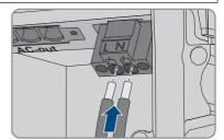
14. Ensure the conductors are plugged into the terminal points (round openings) as far as is will go and not into the actuation shafts (rectangular openings).
