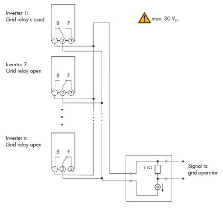
Figure 18: Wiring diagram for signaling the switching status of the grid relay (example)
