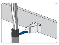
12. Tighten the cable gland. This will provide tightness and strain relief for the communication cable.
