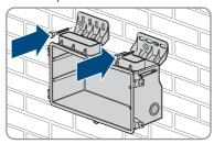
8. Check whether the Connection Unit is firmly positioned.
