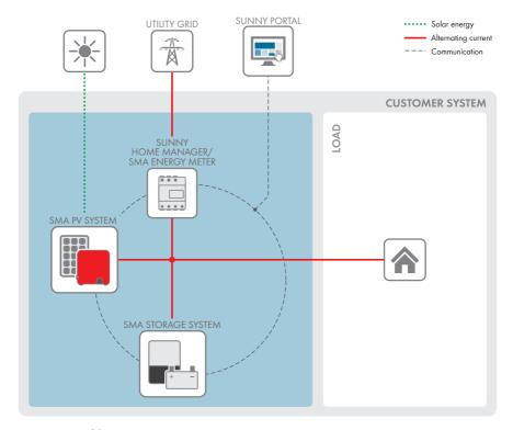
Figure 4: Design of the system
