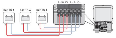
Figure 21: Overview for connection of three batteries with a charging/discharging current limit of 10 A each
