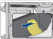
12. Pull the ribbon cable used to connect the communication assembly to the Power Unit into the Connection Unit, and plug it into the jack on the communication assembly.
