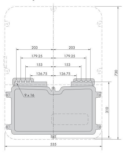
Figure 12: Position of the anchoring points(Dimensions in mm)
