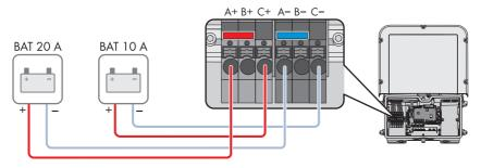
Figure 22: Overview for connection of two batteries with varying charging/discharging current limits
