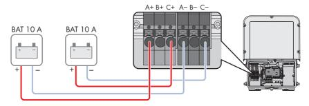
Figure 20: Overview for connection of two batteries with a charging/discharging current limit of 10 A each
