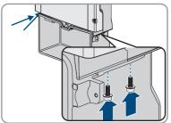
16. Lead the enclosure lid to the Connection Unit and plug the ribbon cable into the socket on the communication assembly.
