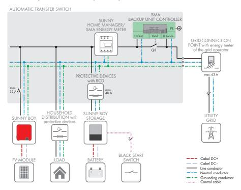
Figure 6: System design of an SMA Energy System Home with battery-backup function (example)
