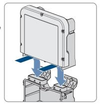
Tighten 2 screws on the right and left side of the Power Unit (TX25) (torque: 6 Nm ± 0.3 Nm).
