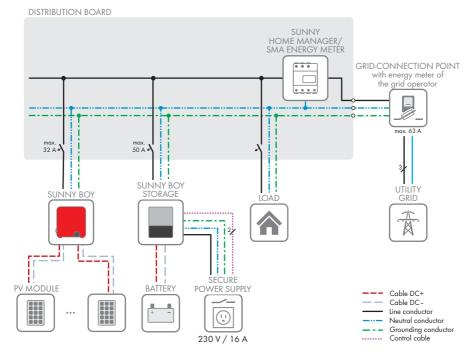
Figure 5: Circuitry overview of an SMA Energy System Home with switch and socket for secure power supply operation (example)
