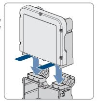
15. Tighten the 2 screws on the right and left side of the Power Unit (TX25) (torque: 6 Nm ± 0.3 Nm).
