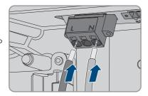
15. Ensure the conductors are plugged into the terminal points (round openings) as far as is will go and not into the actuation shafts (rectangular openings).
