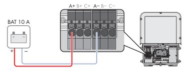
Figure 19: Overview for connection of one battery with a charging/discharging current limit of 10 A
