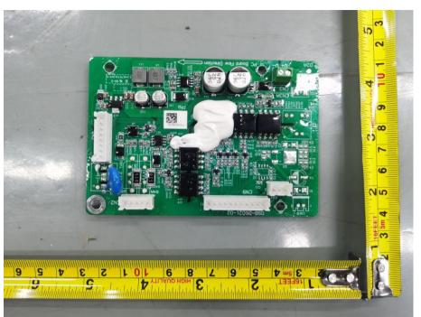
Figure 9. Communication board component side view
