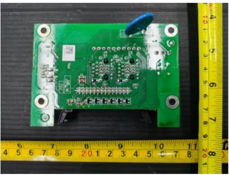
Figure 12. Communication board solder side view
