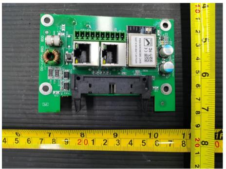
Figure 11. Communication board component side view
