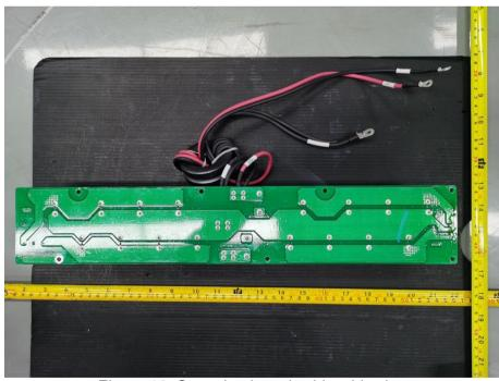
Figure 18. Capacitor board solder side view
