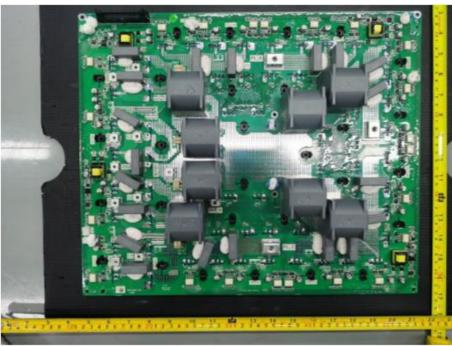
Figure 21. Inverter board component side view
