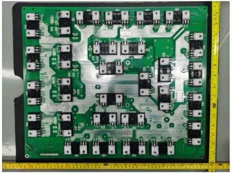
Figure 22. Inverter board component solder view
