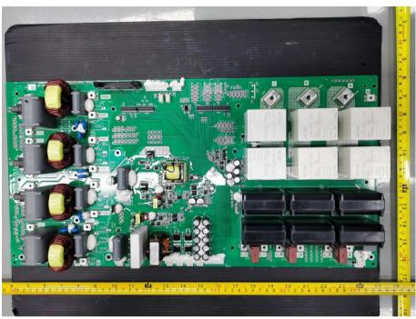
Figure 15. AC board component side view
