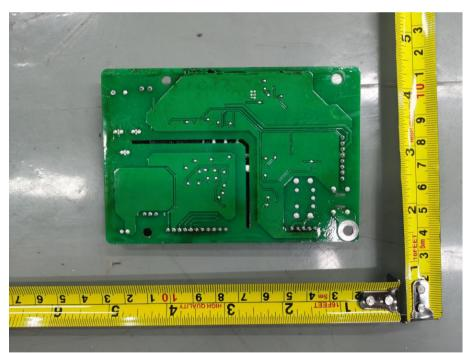
Figure 10. Communication board solder side view
