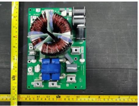
Figure 19. Output board component side view
