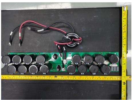
Figure 17. Capacitor board component side view
