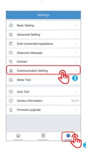
Step 3 (Optional) When multiple inverters are parallel connected, scan the QR code or click <u>Parallel Inverter System Solution User</u> <u>Manual</u> for more details.
